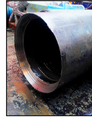
Casing cut by TITAN System
