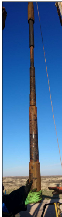
7" PACKER MANDREL AND SLIPS RECENTLY RECOVERED FOR PERMIAN BASIN OPERATOR
