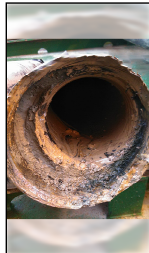
5" & 7" Liner with Settled Barite in Annulus
