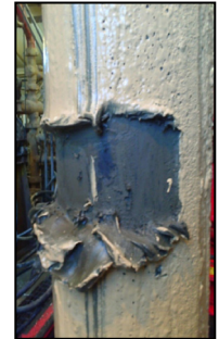
Settled solids covering recovered casing
